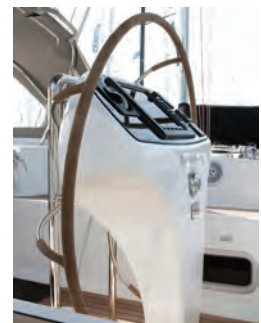
Custom dished wheel designed to mount on the back face of the customer's own pedestal for which they have a registered trademark.
